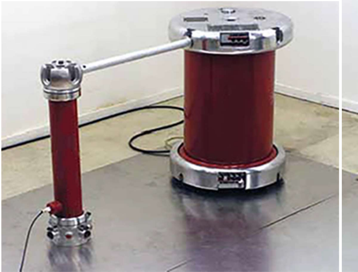
Single-stage AC Voltage Test Set-up
